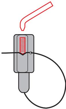
The screw broken in the hole
